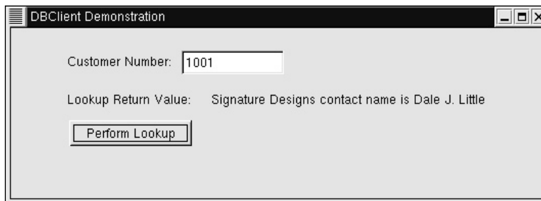
Figure 21-3 The DBClient application uses a TIdTCPClient component to request information from the DBServer application.
