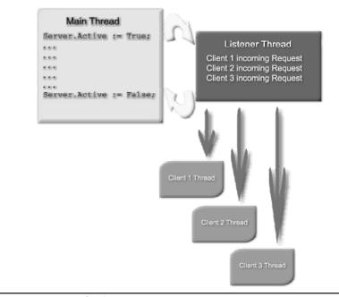
Figure 20-1 Operation of TIdTCPServer
